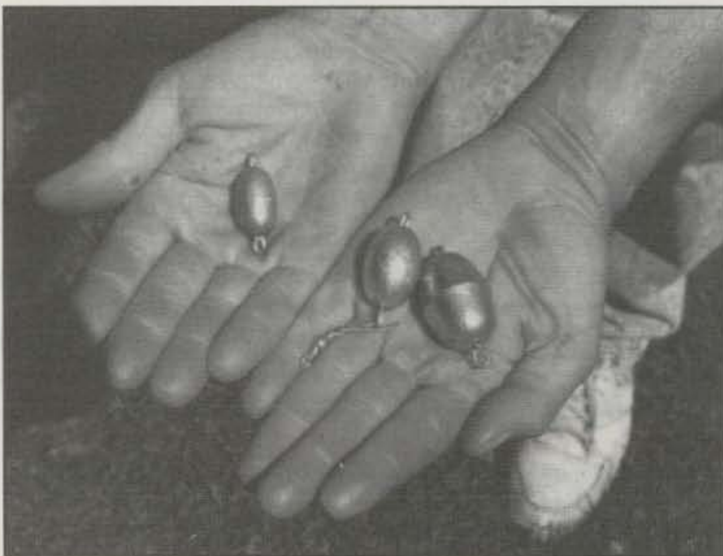
Egg-type sinkers in three sizes weighing 2, 4, and 6 ounces each. A wire has been passed through the hole and eyelets formed at each end. They have been spray painted with aluminum paint. The 4 ounce sinker is equipped with a snap swivel.
